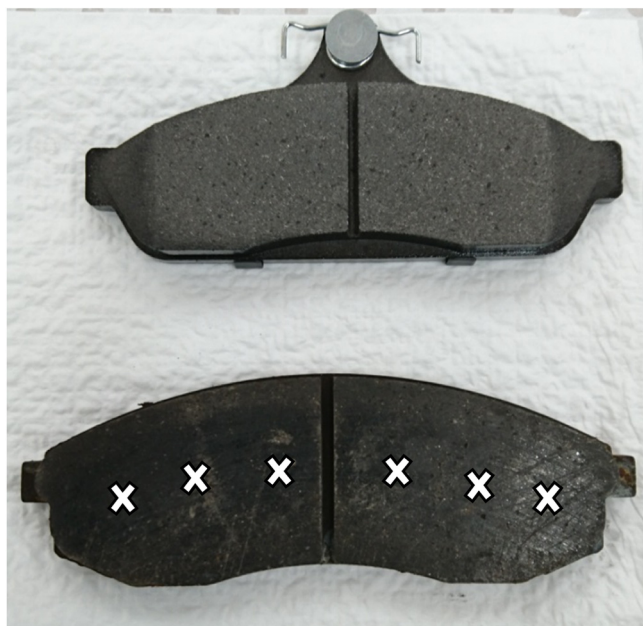
Fig. 1. Exemplar brake pad as used for sampling. Comparison between unworn (top) and worn (bottom) pads. The six points across the surface of the pad analysed by XRF are designated with an 'x'.
