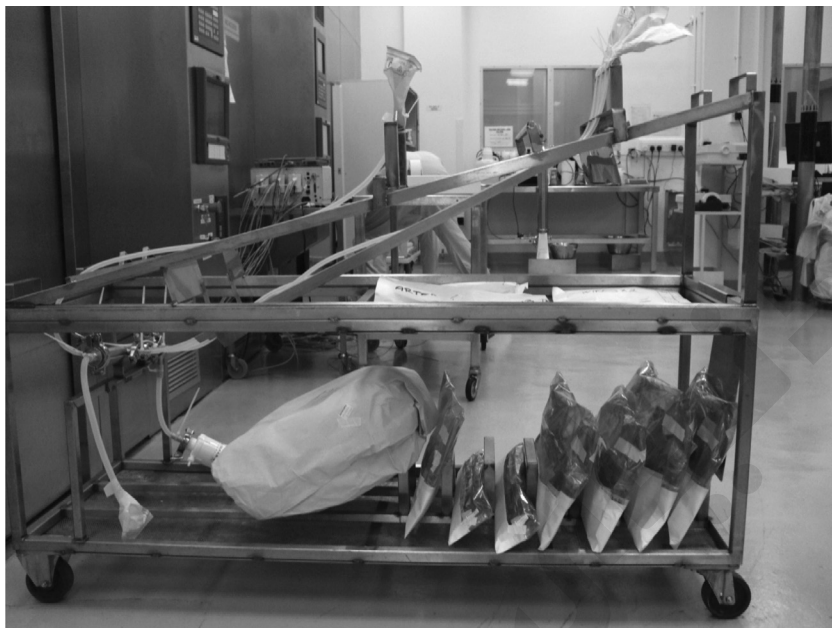
Figure 7.2 Typical autoclave load at a pharmaceutical facility
