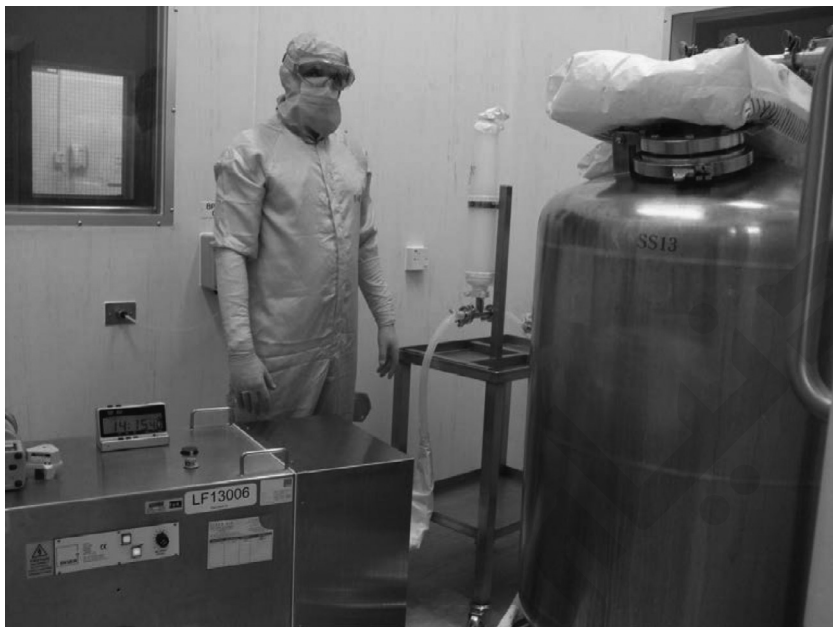
Figure 15.1 Liquid media being filtered in for a media trial
