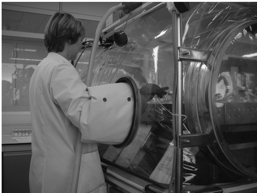
Figure 13.3 An operator preparing a flexible film isolator
