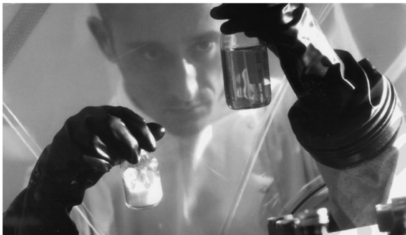
Figure 19.2 Inspecting Sterility Test media for turbidity
