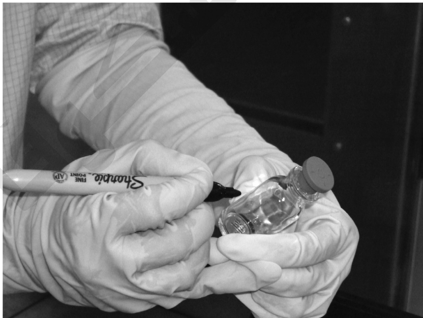
Figure 12.2 A depyrogenated glass vial complete with rubber closure
