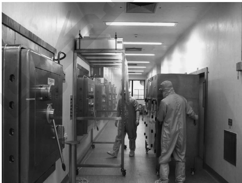
Figure 15.2 Loading a lyophiliser
