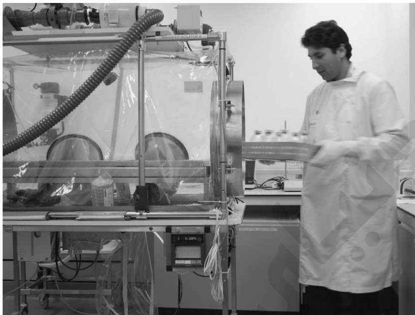
Figure 14.2 Operator loading a flexible film isolator in a laboratory
