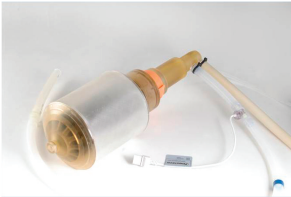
Figure 9.6 The single-use module from a CARR Centritech closed, continuous bioprocessing capable centrifuge.
