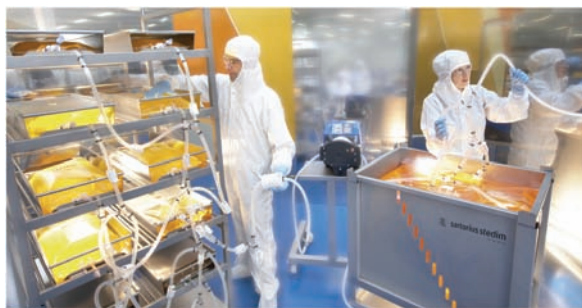
Figure 16.2 Large volume to small volume transfer (courtesy Sartorius Stedim, Inc.).
