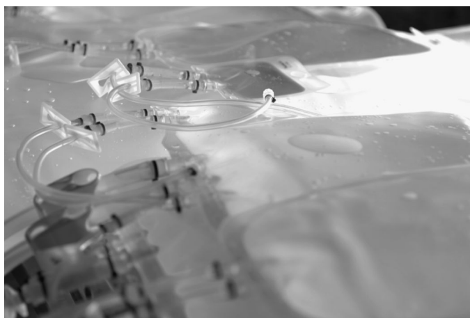
Figure 9.3 Continuous biomanufacturing capable Thermo™ Scientific™ BioProcess Container assembly.
