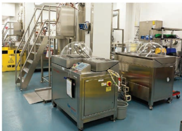
Figure 18.2 Continuous centrifugation units used for a perfusion process (from Ref. [18]). Copyright 2012 held by Shire with all rights reserved. No party may make any use of this image without the express written permission of Shire.
