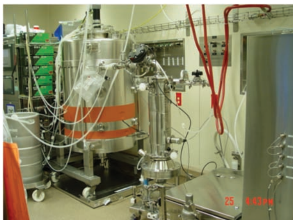
Figure 18.3 Alternating tangential filtration (ATF) unit connected to a 500l bioreactor used for a perfusion process (from Ref. [15]).
