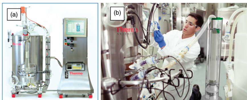
Figure 9.4 Single-use, perfusion bioproduction accomplished in a single-use Thermo Scientific HyPerforma S.U.B. TK 250L (a) depicted with a Refine Technology single-use ATF6 System (b).
