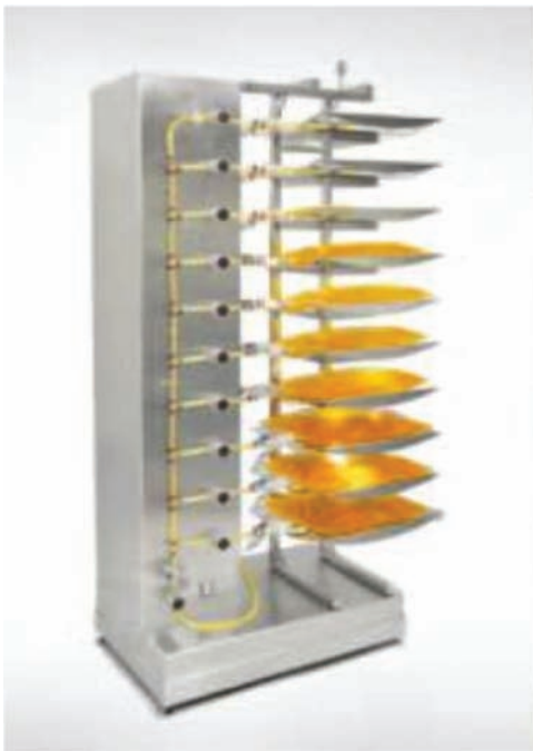
Figure 16.6 Automated fill system, portion large volumes (courtesy of Sartorius Stedim).
