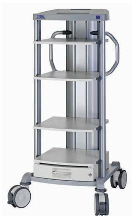
UG120 **Equipment Cart**, narrow, high, rides on 4 antistatic dual wheels equipped with locking brakes, mains switch on cover, energy beam with integrated electrical subdistributors with 12 sockets, potential equalizer connectors,
