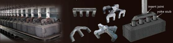
this company has a special plant and exclusive method and analysis to produce Rods and joint to yoke with the latest world wide method. In addition the company can stablished industrial site in distonation country to joint Rod and yoke Or can export complete Anode yoke directly from origin.
