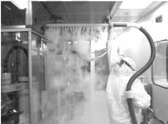
Figure 1: Example of ducted smoke through a perforated pipe in order to obtain a curtain-like effect.
