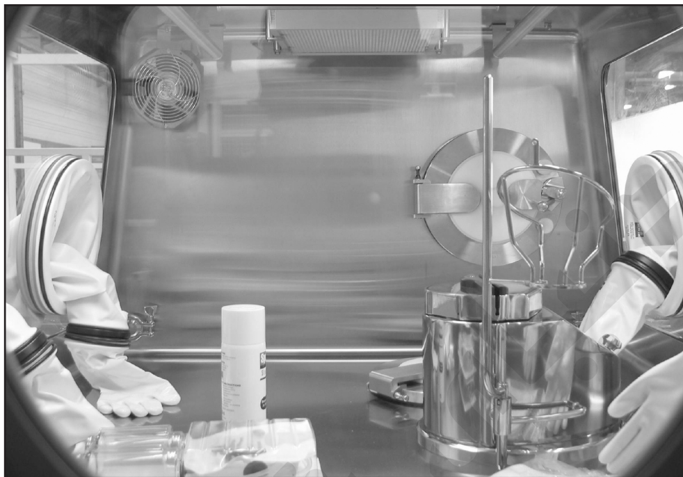
Figure 7: A sterility testing isolator (courtesy of Getinge).
