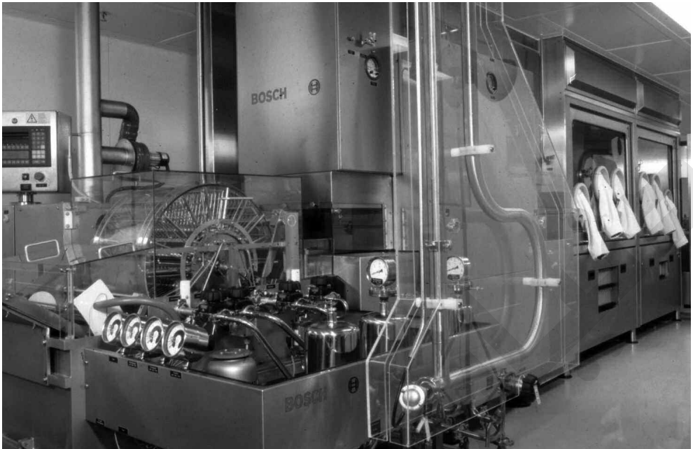
Figure 8: Isolator protected ampoule filling machine (Copyright: Cilag AG, CH-8201 Schaffhausen, image courtesy of Schicht Hans H.: 40 years of cleanroom technology – some historical remarks. In: Proceedings of the 17th International Symposium on Contamination Control, Bonn, Germany, 6-9 Sept. 2004 , p. 1-10. Edited by: Verein Deutscher Ingenieure (Association of German Engineers), Düsseldorf, Germany 2004.
