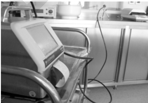
Figure 18: Typical particle counter and display screen.
