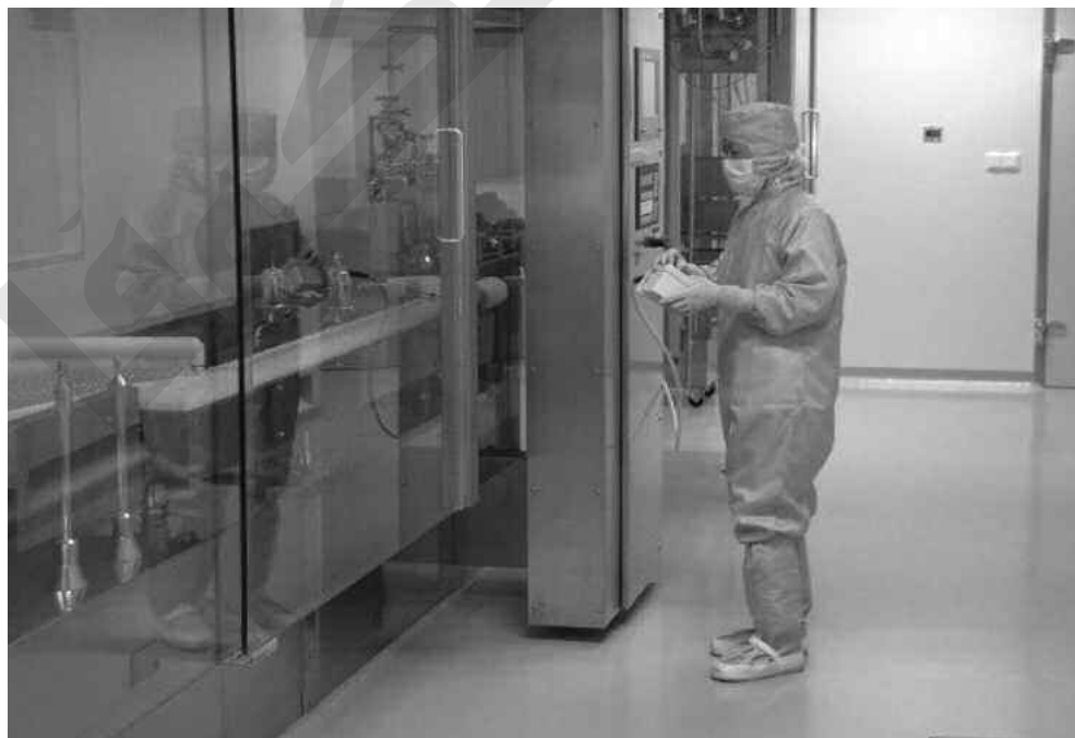
Figure 3: Cleanroom and critical workstation used for aseptic preparations.
