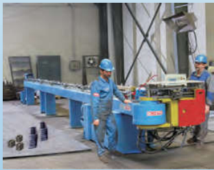
Three Unit Tube Bending Machine OD up to 4"
