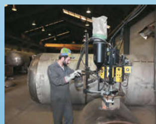
Automatic Circle Welding On Pipe and Pressure Vessel From 2" OD Up to 24"
