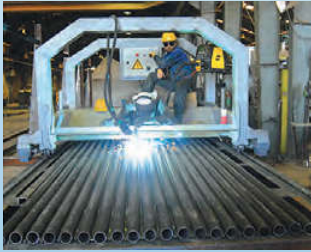
Automatic Panel Membrane Wall Welding Machine
