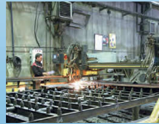
ESAB - CNC Plasma & Oxy Cutting Machine 14000mm x 4000mm
