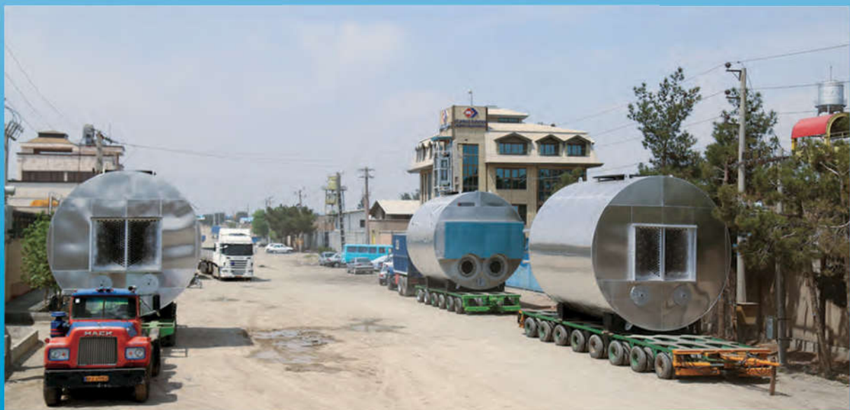
Three Condor Twine furnace steem boilers on skids for transpant each boiler suturated steem flow Rate 60,000 lb/hr for Caspian Paper Co.
