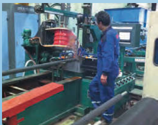
High-frequency Welded Finned Tube Machine Solid and serrated fin Tube diameter up to 219 mm Tube length up to 16000 mm
