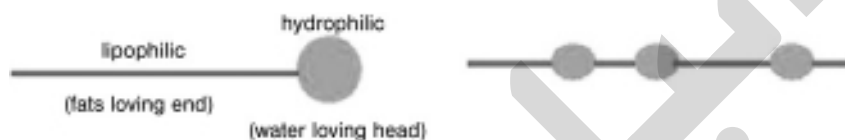
Figure 5.3 Basic structure of surface active agents.
