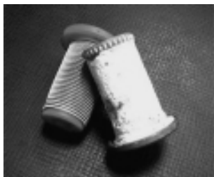
Figure 7.24 Calcium soap precipitation due to sub-stoichiometric ratio between EDTA and water hardness.
