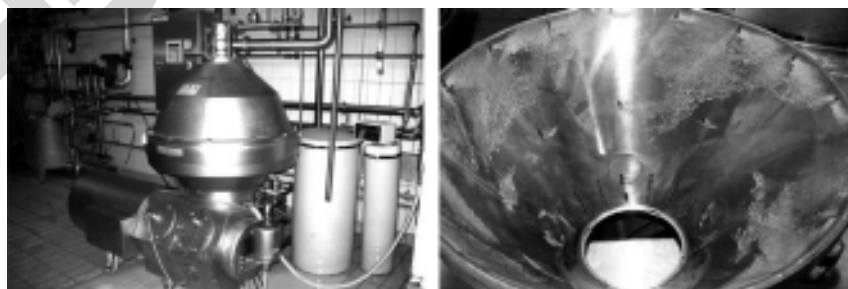
Figure 8.20 Separator and example of incomplete cleaning.
