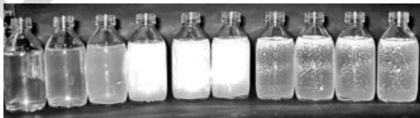
Figure 7.37 Dispersed and coagulated oleic diamine-sulfate salt.
