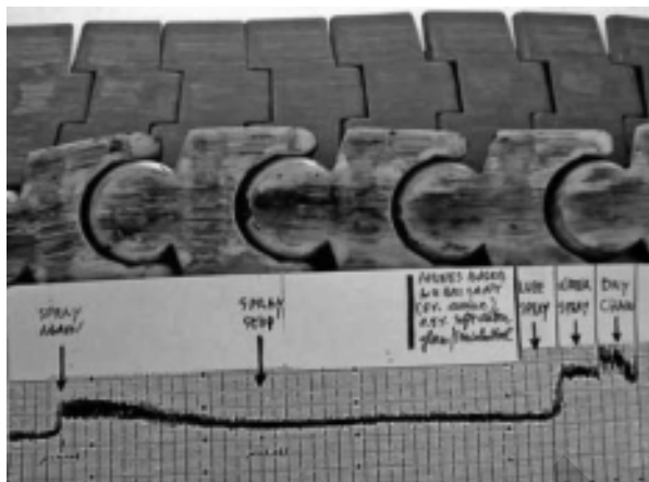
Figure 7.14 Tracks are always damaged in the absence of lubricant.
