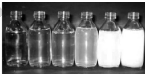
Figure 7.36 Oleic diamine 200ppm in water. Concentrations of sodium sulfate up to 1000ppm. PH 6.8 with acetic acid. The picture relates turbidity to absorption.
