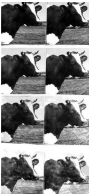
Figure 7.27 Paint fading by excess of surfactants.
