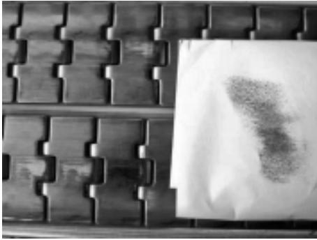
Figure 7.8 Oily deposit containing black oxides.
