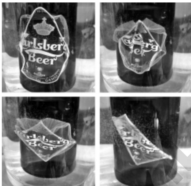
Figure 6.19 Experimental thermoplastic labels (courtesy of Steinbeis Co. and Simonazzi).
