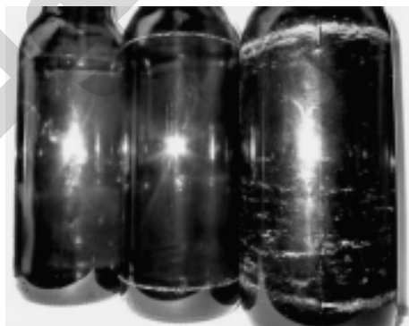
Figure 6.36 Scuffing in the life of a bottle.
