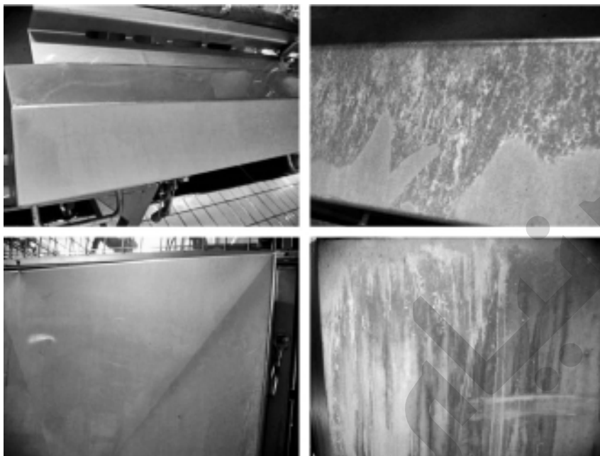
Figure 11.9 Cleaning problem from unsuitable concentration of detergent.
