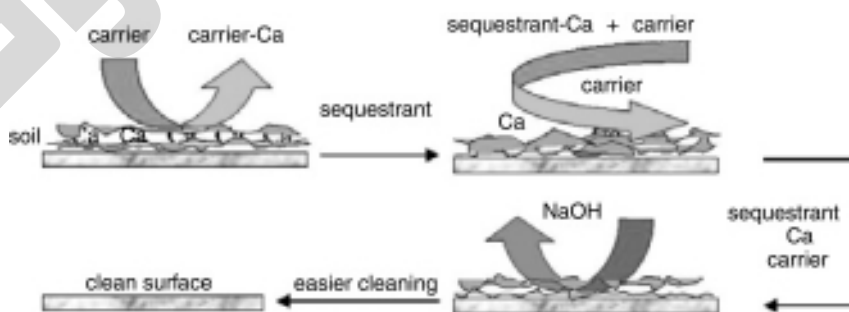
Figure 3.5 The carrier mechanism of sequestrants makes the cleaning easier.
