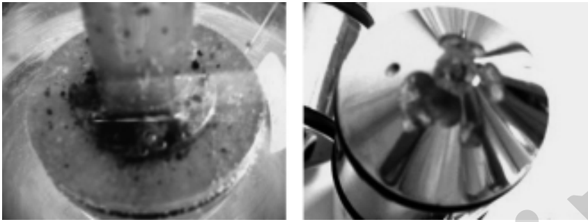
Figure 17.12 Pitting corrosion from chlorinated detergent.
