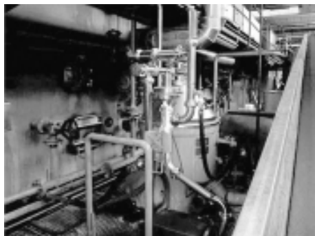
Figure 6.34 Centrifuge added to the caustic bath in mineral water bottling.
