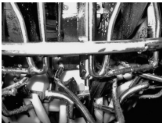
Figure 11.11 Cleaning problem from unsuitable temperature or worker negligence.
