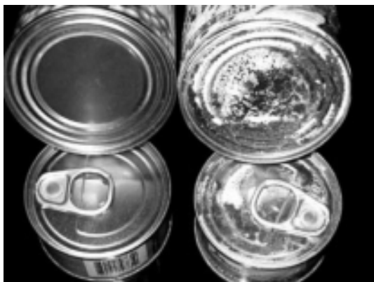
Figure 8.29 27 dF hardness and 100ppm of sequestrants: comparison between citric-tartaric acid and hexametaphosphate-ATMP.
