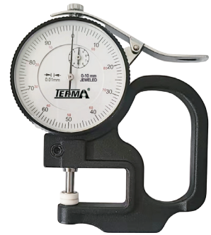
Dial Thickness Gauge 0-10mmx30mm
