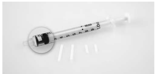
Figure 10 Spore strip biological indicator placed inside syringe.
