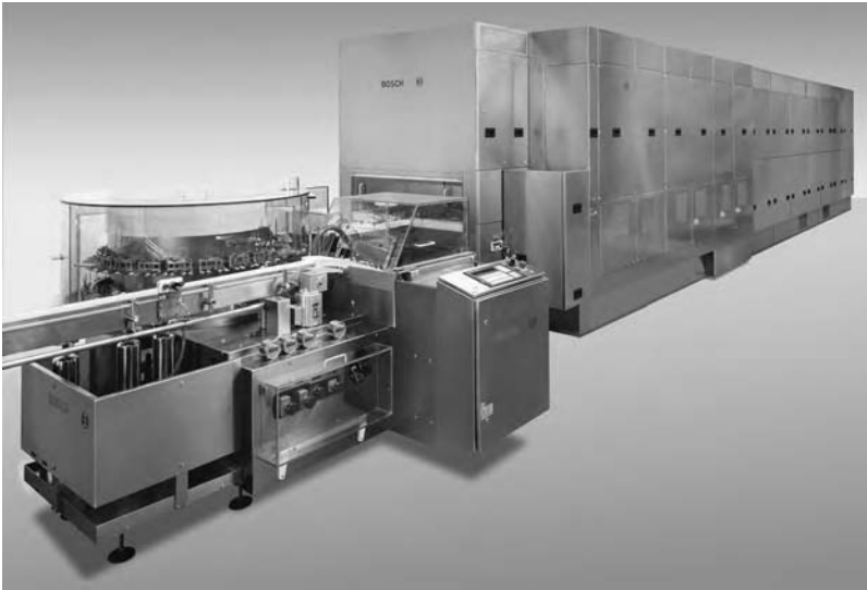
Figure 3 A commercial depyrogenation tunnel with vial washer. (HQL 5000 Series Depyrogenation Tunnel with RRU Vial Washer). Source: Courtesy of Bosch Packaging Technology Inc., Minneapolis, MN.
