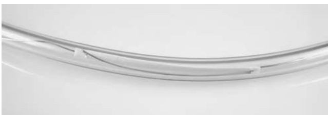
Figure 9 Spore strip biological indicator placed inside process tubing.
