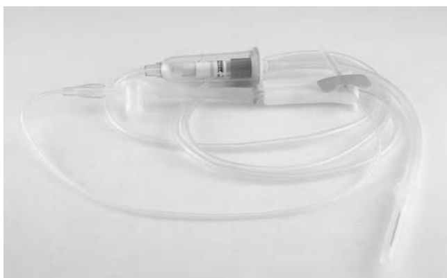
Figure 11 Self-contained ethylene oxide biological indicator placed inside the IV drip chamber of a drug administration set.
