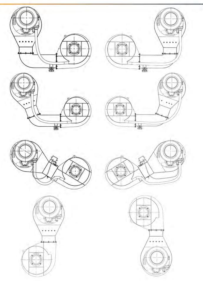
According to the dimensions and design of the boiler, the burner can be installed at different angles.
