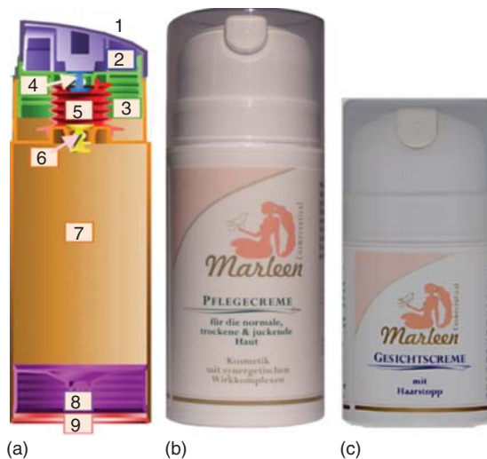
Figure 13.32 Airless dispensers: (a) explanation of the function via the cross section: (1) cap (PP), (2,3) head (PP), (4) upper valve (EVA, ethylene vinyl acetate), (5) bellows (LD-PE), (6) lower valve (POM, polyoxymethylene), (7) container for
