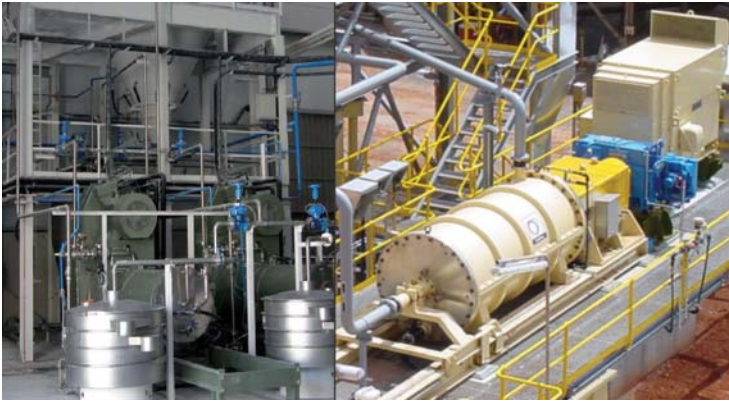
Figure 7.13 Grinding plants in production (a) milling of calcium carbonate in two 500 l mills; and (b) large bead mill for minerals and ores (Courtesy of Netzsch).
