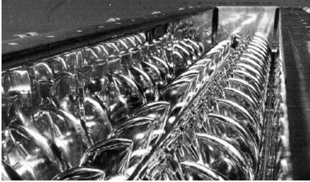
Figure 16.2 Large twin-shaft mixer with clean surfaces, polished to a mirror finish on walls, shafts, and tools (Courtesy of Nara Machinery Co., Ltd. Europe).
