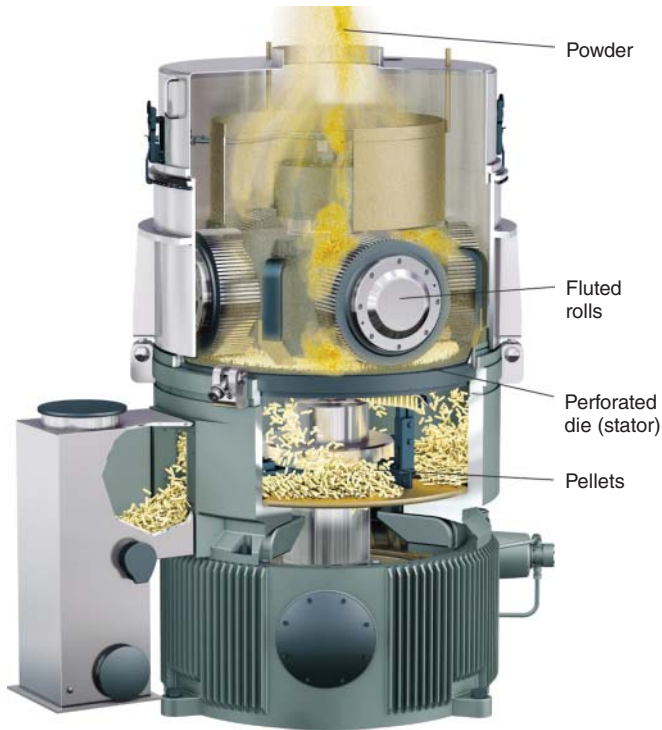
Figure 5.6 Pelleting machine with moving rollers on an annular flat die (Courtesy of Amandus Kahl).
