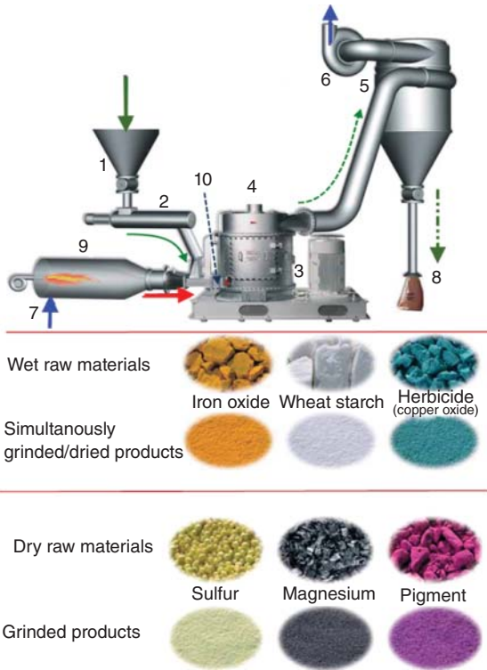
Figure 7.16 Plant for grinding, mill drying of moist solids and of pastes; 1: container for (moist) raw materials; 2: dosing screw for feeding the solids; 3: air turbulence mill; 4: integrated classifier; 5: product filter;
