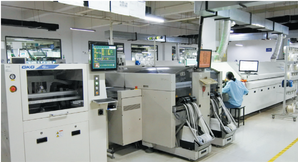
• Germany-made Siemens SMD - 3 lines of D4i and D1 surface mounting devices
