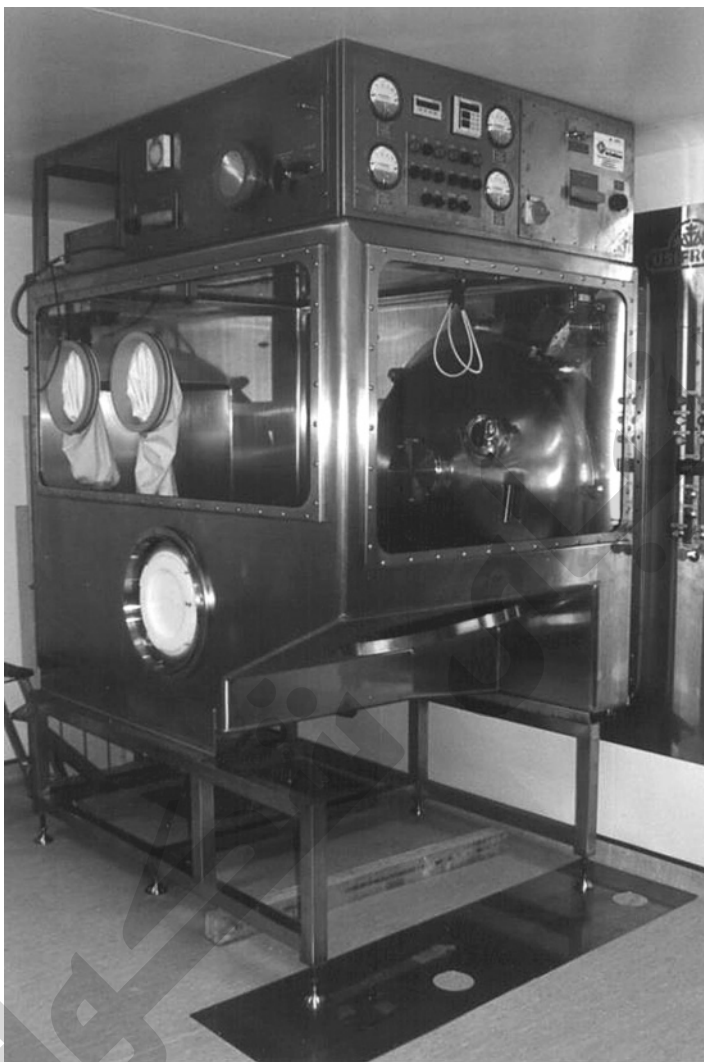
Figure 10.15 The Freeze-Dryer Isolator. The half-suit has been removed so that the door of the drier can be clearly seen in this view. It hinges into a recess on the back face of the isolator, opposite the half-suit plinth.
