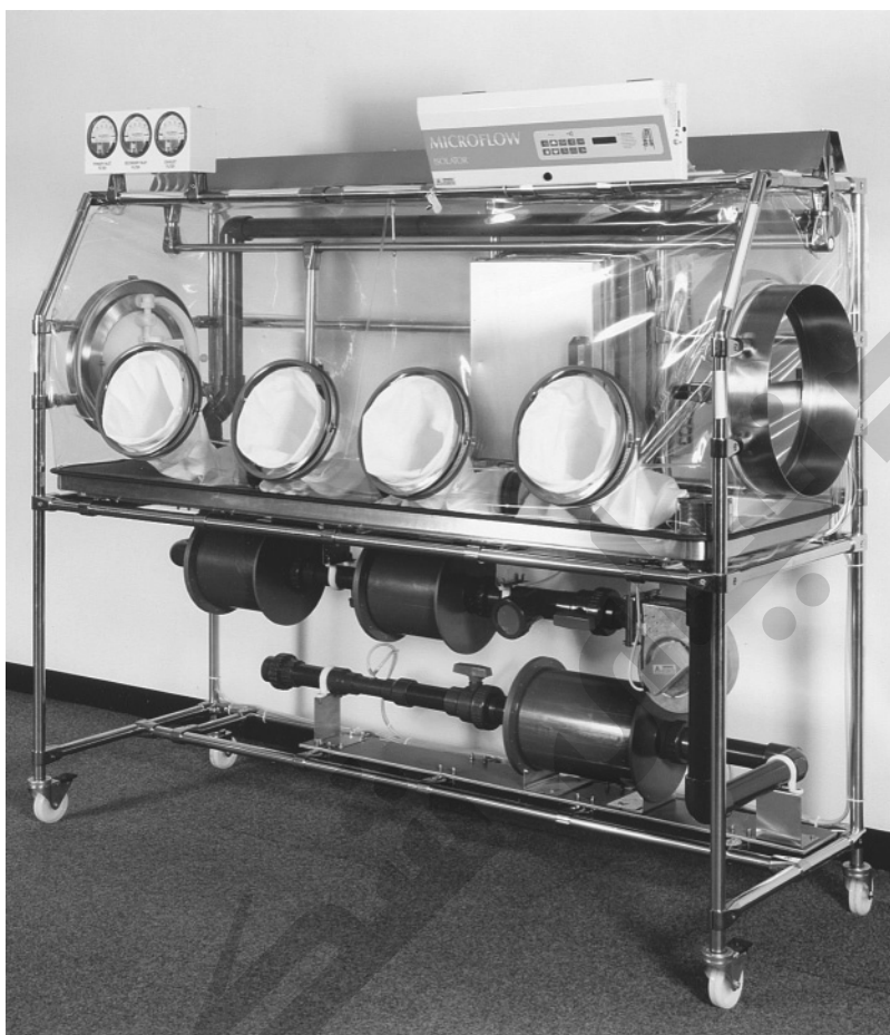
Figure 1.2 A Four-Glove Flexible Film Isolator. This isolator forms part of a suite used for aseptic dispensing in a large hospital pharmacy and is used as a sterile bank, storing materials ready for dispensing in other smaller isolators. Note the RTP on the left-hand end and the refrigerator fitted to the back wall of the isolator. (Courtesy of Astec Microflow.)
