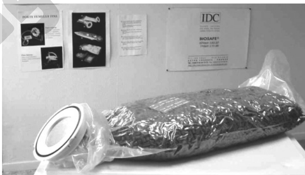
Figure 3.16b An IDC BioSafe Container with Male or Beta Flange. This container is designed to hold presterilised stoppers. (Courtesy of IDC.)
