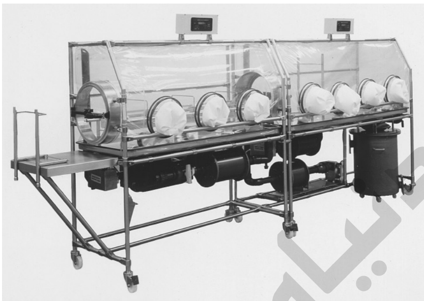
Figure 1.3 A Flexible Film Isolator System Used for Sterility Testing in a Blood Product Laboratory. The left-hand isolator is used to sterilise and transfer materials through to the working isolator on the right. Note the “railway” system used to move sample trays easily through the isolators, and the RTP wastebin underneath the working isolator. (Courtesy of Astec Microflow.)
