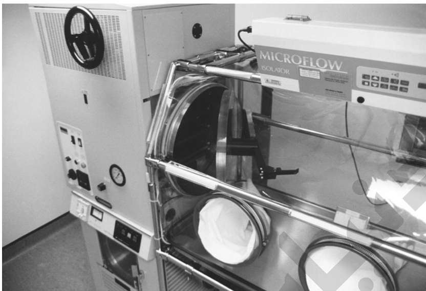
Figure 3.24 A Pilot-Scale Installation of a Glove Isolator and a Small Freeze Dryer. Note how the door of the freeze dryer opens out into the isolator. (Courtesy of Astec Microflow.)
