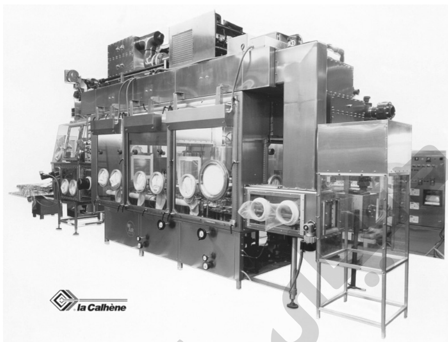
Figure 3.21 A Complete Filling Line Isolator System. This photograph shows some of the technical complexity that may be required with such installations. (Courtesy of La Calhène SA.)
