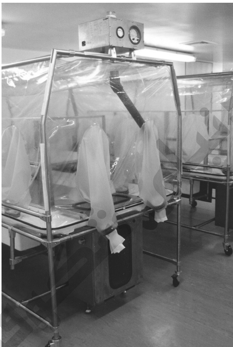
Figure 2.10 Natural PVC Sleeves Welded in to Form Part of the Canopy on a Bio-medical Isolator. (Courtesy of Astec Microflow.)
