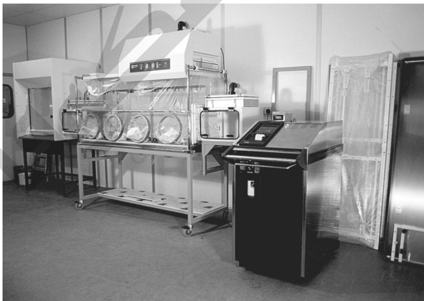
Figure 7.8 The Steris VHP 1000 Hydrogen Peroxide Gas Generator in Use with a Flexible Film Isolator. (Courtesy of Envair Ltd.)
