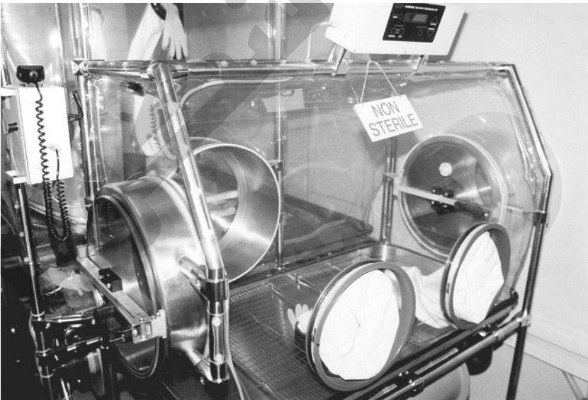
Figure 10.2 Detailed View of the Glove Isolator. A more detailed view of the glove isolator with connection to the main half-suit isolator and also through the wall to another room. (Courtesy of Aventis.)
