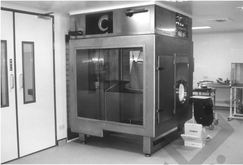
Figure 10.9 The Depyrogeneration Oven Isolator. The carriage moves out of the oven to occupy the space immediately in front of the half-suit operator. The loading end of the oven is accessed from the preparation area, which is located through the double doors on the left.
