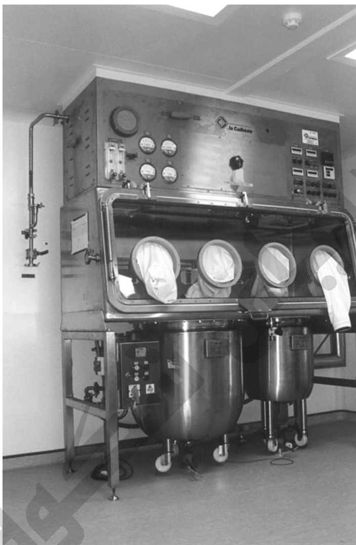
Figure 10.8 The Compounding Isolator. Note the 200-litre and 60-litre vessels mounted under the floor. These are fitted with wheels to aid removal during major cleaning, but are normally jacked up to seal against the floor of the isolator.
