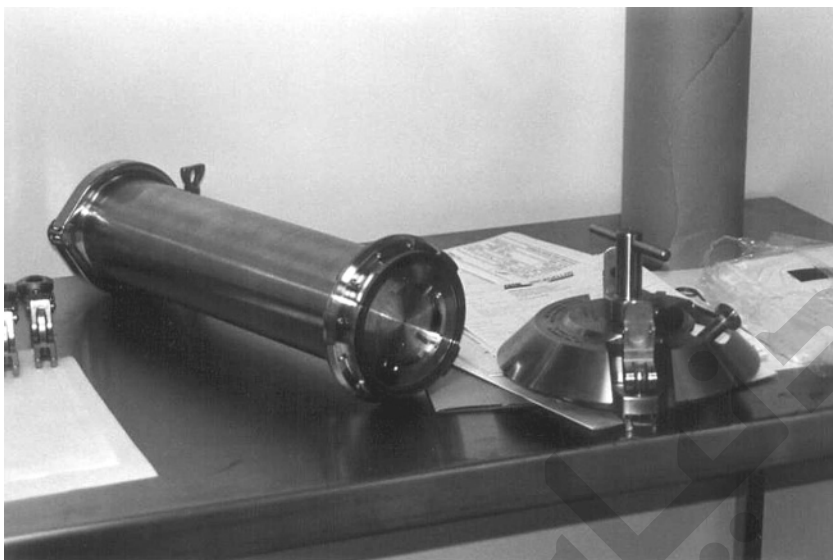
Figure 10.14 An SIP RTP Container as Used for Making Aseptic Connection between the Mobile Product Vessels and the Filling Isolator. The flying saucer-like object fits onto the container during SIP, allowing the lid to be lifted and thus getting steam to the occluded surfaces of the lid assembly.
