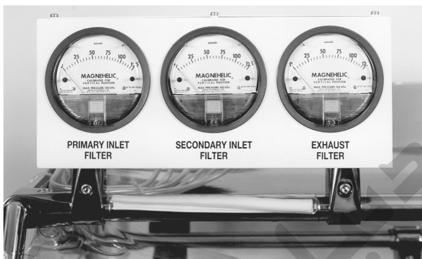
Figure 4.4 Gauges Fitted across HEPA Filters on a Flexible Film Isolator. The gauges show their condition. The client chose to fit double inlet filters in this application for added sterile product security. (Courtesy of Astec Microflow.)
