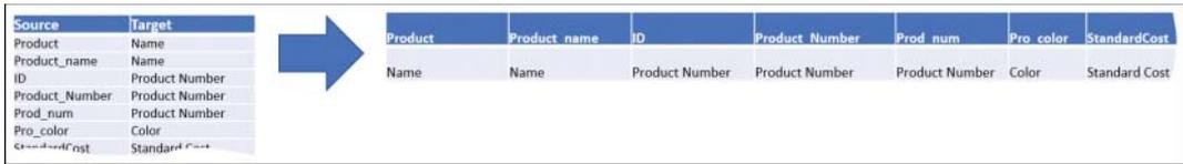
**FIGURE 4-11** Transposing the original conversion table of Source/Destination pairs into a single-row table can be an efficient method of normalizing the column names.
