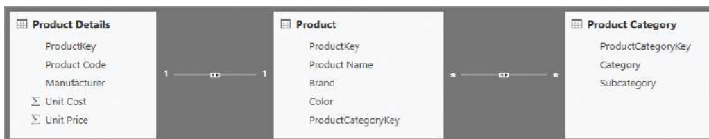
FIGURE 14-2 In this model both relationships have a bidirectional filter. One relationship is one-to-one, and the other is many-to-many.
