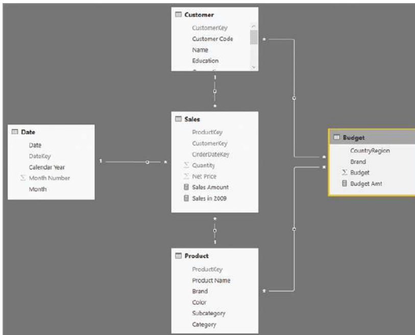
FIGURE 15-24 Budget is directly linked to Customer and Product using two weak relationships.
