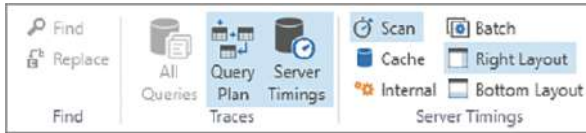
FIGURE 19-9 The Query Plan and Server Timings options enable the tracing features in DAX Studio.
