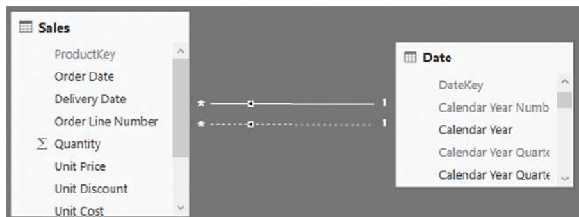
FIGURE 15-33 No more than one relationship can be active between any two tables.
