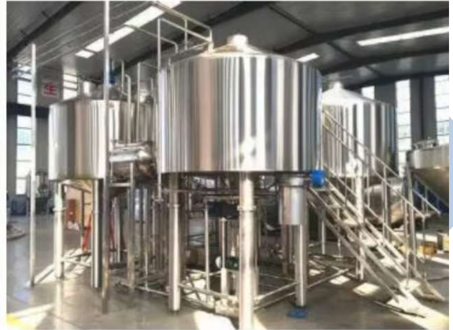
30HL 4 vessels brewhouse:mash+lauter+kettle+whirlpool
